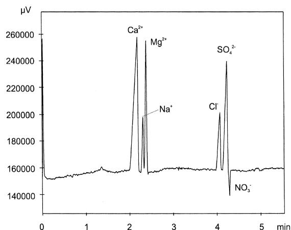
Fig. 4. Simultaneous determination of cations and anions in drinking water (dilution 1:20). Injection: hydrodynamic (10 cm for 10 s at the anodic end and 10 cm for 5 s at the cathodic end; other conditions see Fig. 3).
