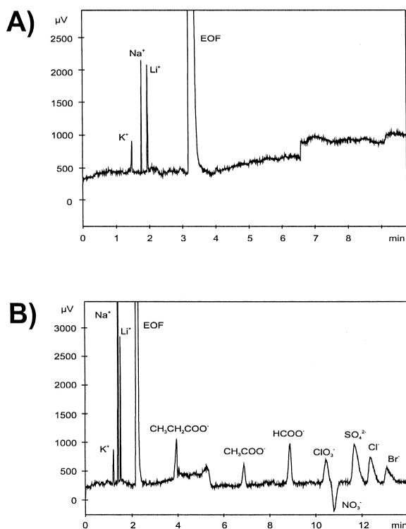
Fig. 2. Electropherograms of simultaneous cation and anion separation. (a) Separation by utilization of the EOF (b) Separation with electrolyte flow generation by external pressure (pressure application of 200 mbar at the anodic end of the capillary) Conditions: electrolyte: 5 mM imidazole, 5 mM thiocyanate; capillary: fused-silica 60 cm total length  $\times$  75  $\mu$ m I.D.; detection: indirect UV detection (220 nm); separation: 30 kV; injection: 50 mbar, 10 s.
