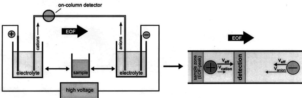
Fig. 1. Principles of the simultaneous determination of cations and anions.
