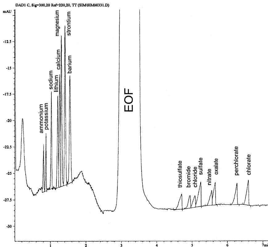
Fig. 7. Simultaneous determination of cations and anions using the DIPP–TMA system. Capillary: fused-silica, 15.5 cm from the anodic and 60 cm from the cathodic end of the capillary to the detector, 75  $\mu\text{m}$  I.D.; other conditions see Fig. 6.
