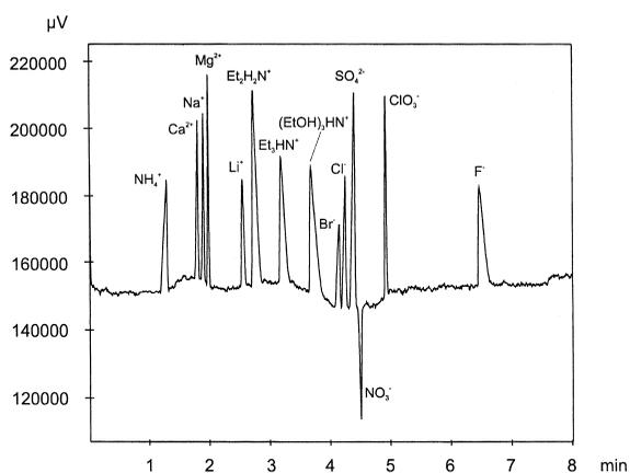
Fig. 3. Electropherogram of a simultaneous cation and anion separation using the imidazole–thiocyanate system. Electrolyte: 5 mM imidazole, 5 mM thiocyanate, 2 mM citric acid, 1 mM 18-crown-6; capillary: fused-silica, 16 cm from the anodic and 50 cm from the cathodic end of the capillary to the detector, 50  $\mu\text{m}$  I.D.; detection: indirect UV detection (220 nm); separation: 30 kV; injection: electrokinetic 3 kV, 10 s.
